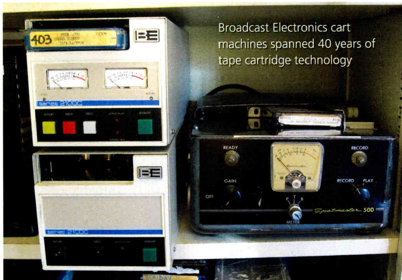
Spanning the years, two Broadcast Electronics 2100C models, left, with their later-generation integrated circuits and precision tape transport, sit side by side with a Spotmaster 500, built with transistors and vacuum tubes.
