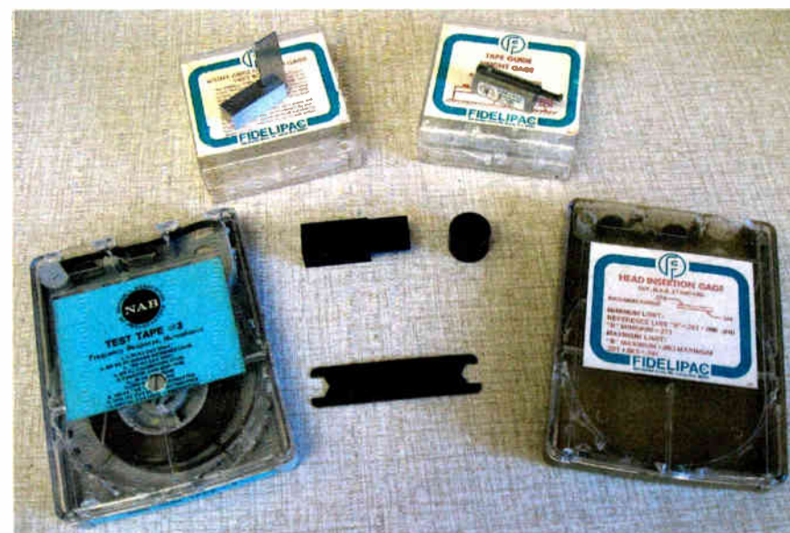
Tools used to align the cart deck evolved over the years, from the simple head alignment wrench, center front, to more precision devices like the right angle zenith and tape guide height gauges made by Fidelipac.
