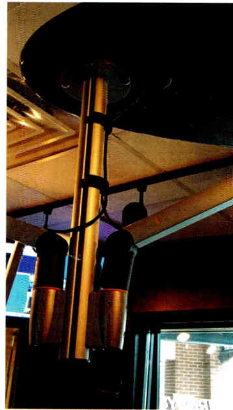
Fig. 2: Standard mic mounting and monitor hardware is used, only inverted!
