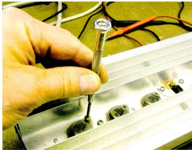
Fig. 5: Use a jeweler's screwdriver to start bolts.
