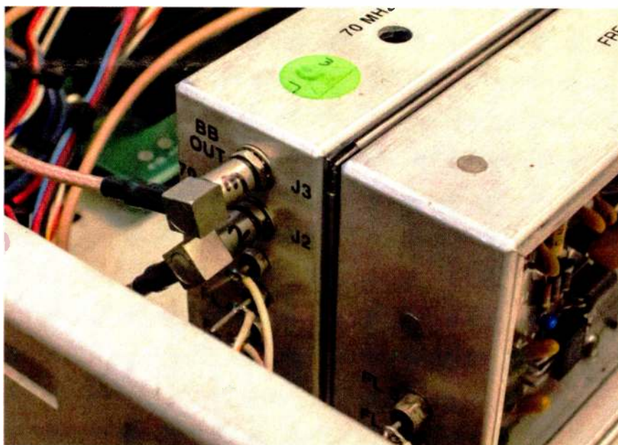
Fig. 2: Label connectors to avoid errors.
