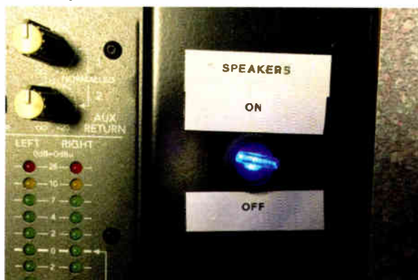
Fig. 2: A switch, tied to a multiple-pole relay like Henry's Superelay, can mute the speakers simultaneously.
