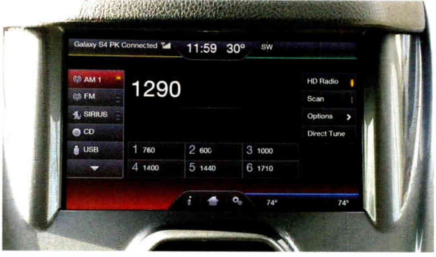
This is how an AM station display appears in Sync with MyFordTouch.
