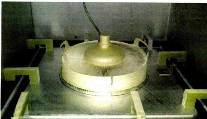
Fig. 2: Here's a 4CX20,000D tube in a Harris FM transmitter.
