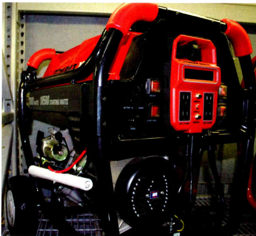
This generator can easily power a 1–2 kW transmitter and is inexpensive, but lacks auto-start and a changeover switch.
