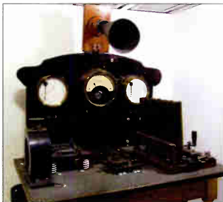
In 1906 the first radio transmission of speech was performed using a sound-modulated arc transmitter. Photo from the Deutsches Museum.
