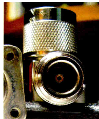
Fig. 3: This is a 50-ohm N connector in a right-angle configuration. Again, note the center female receptacle "pin" diameter, compared to Fig. 2.
