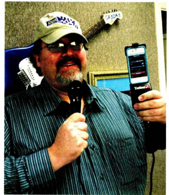
The author's smartphone rests in the Tieline Mic Adapter; a handheld mic is connected and provides audio. The codec can be seen on the phone screen. It feeds audio to the station or can record it.
