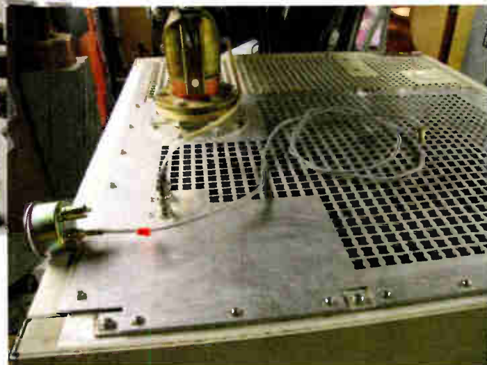
Fig 2: The interconnecting cable is coiled atop the transmitter and needs no plastic tie-wraps.
