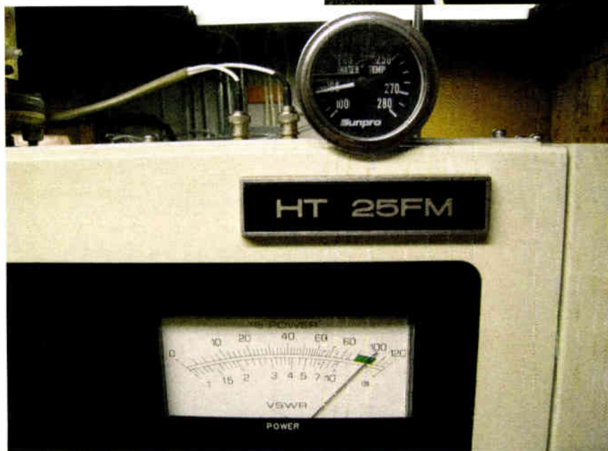
Fig 3: You can easily compare the correlation between temperature and transmitter efficiency by locating the temperature meter near the transmitter PA meters.
