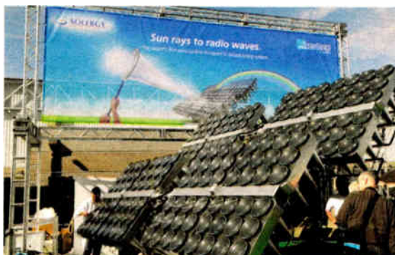
Solergy makes a Cogeneration Concentrated Photo-voltaic solar energy system, or Co-gen CPV, that promises very high efficiency.
