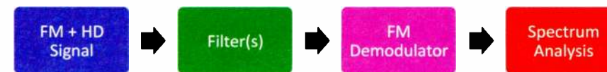
Fig. 8: Complex baseband simulation. The FM demodulator includes a hard limiter and produces FM(t) = Q(t) \times \frac{dI}{dt} - I(t) \times \frac{dQ}{dt} as the demodulated FM.
