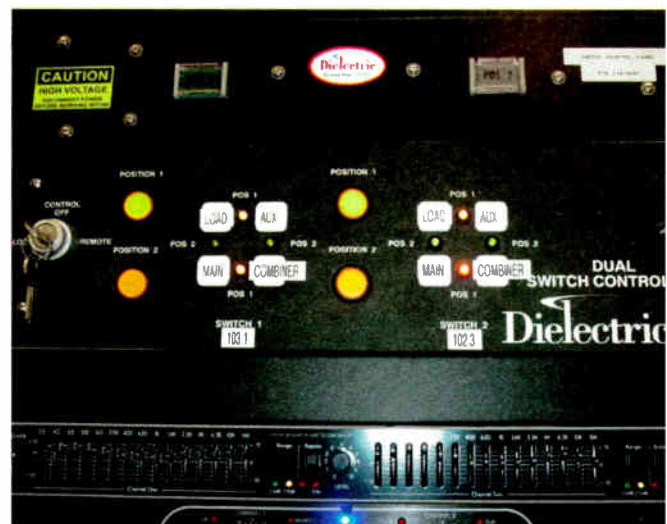
Fig. 2: A 'smart' antenna controller, properly wired, ensures against damage caused by hot switching.
