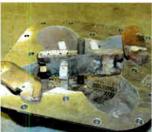
Fig. 4: Inside a burned RF switch. RF has no mercy. Wire those interlocks.
