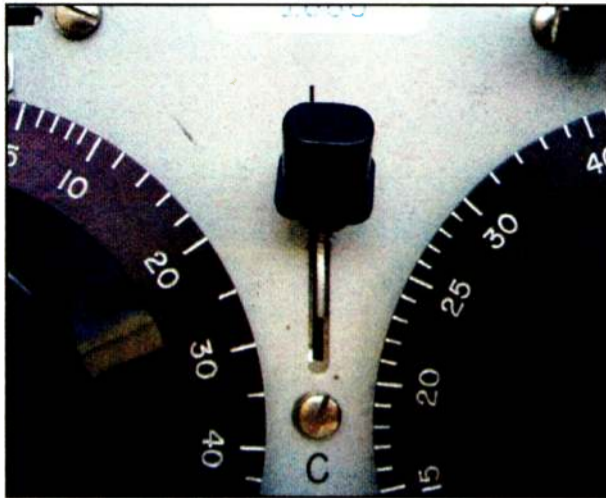
Fig. 1: An OIB is used to measure impedance under actual operating conditions.
