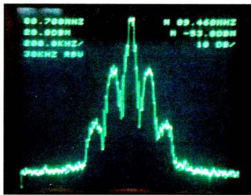
Fig. 5: Spectrum Analyzer Capture of a System With 'Grunge'
