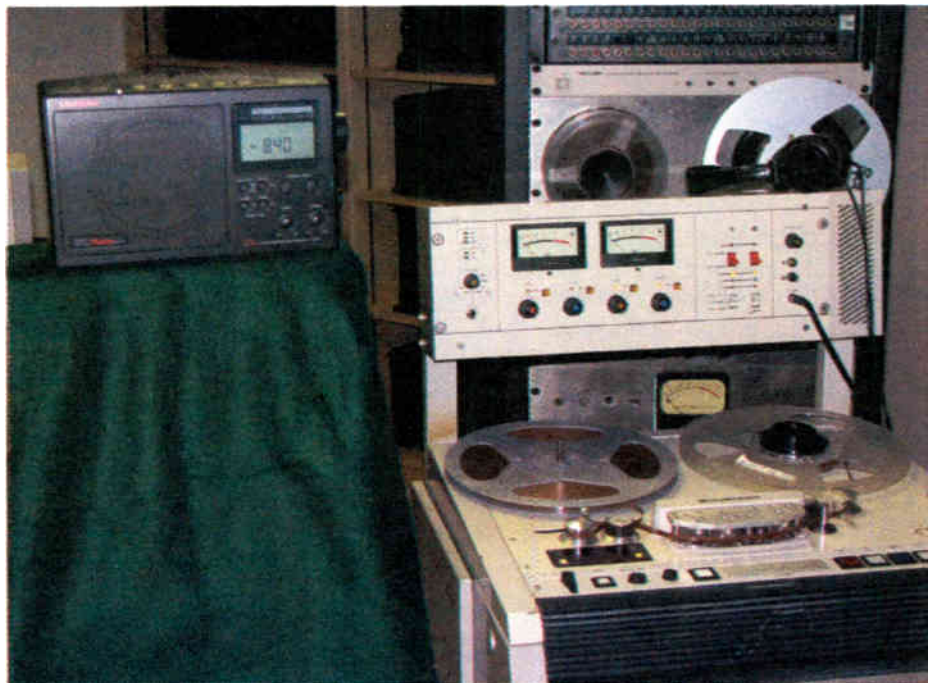
The Sangean radio is tuned to WHAS, Louisville, Ky., at 840 kHz. Alongside is one of the author's Otari MTR-10 audio recorders used to record 'before/after' audio and a rack-mounted Tascam LA-40 unbalanced/balanced audio converter to feed audio from the radios to the Otari.
