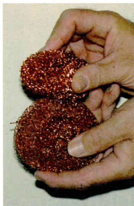
Fig. 2: As a replacement for copper wool, use less expensive stainless steel wool to plug holes.
