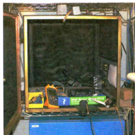
Radios are isolated in this screen box for testing.
