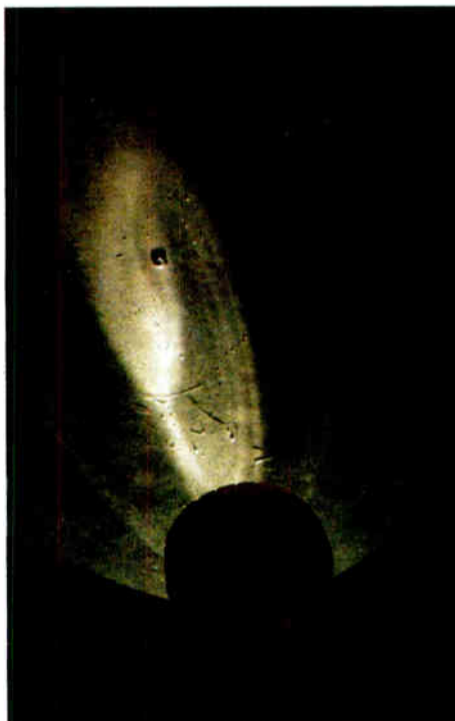
Fig. 2: Oh, there it is! Shine a flashlight parallel to the floor to locate dropped hardware.
