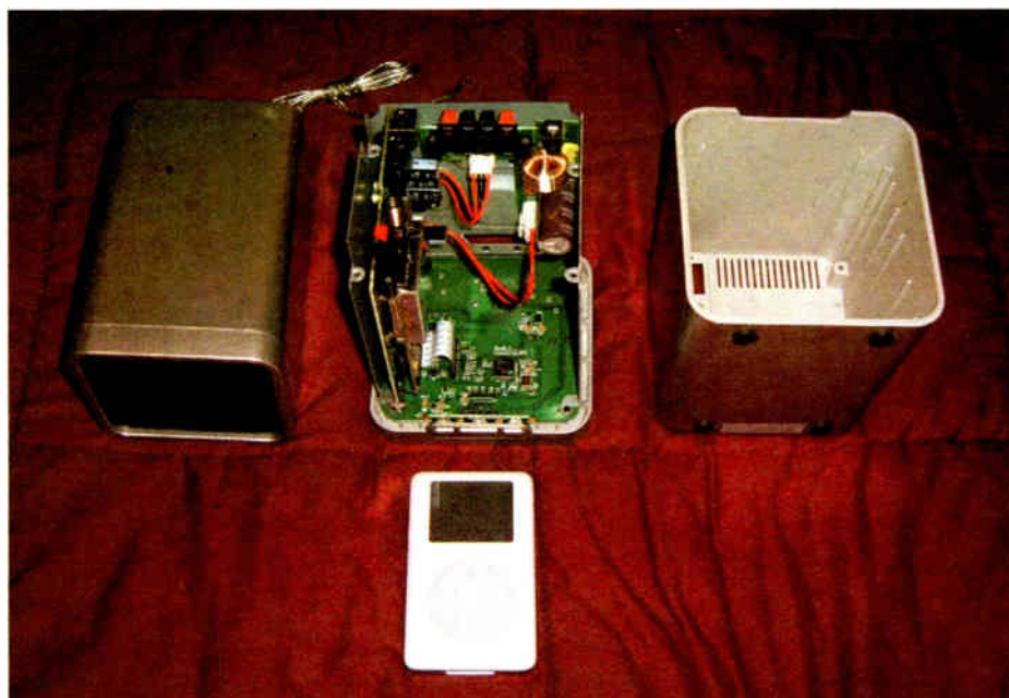
Removing eight screws from the rear reveals a sparse interior. Most of the electronics are packed along the front, bottom and one side.
