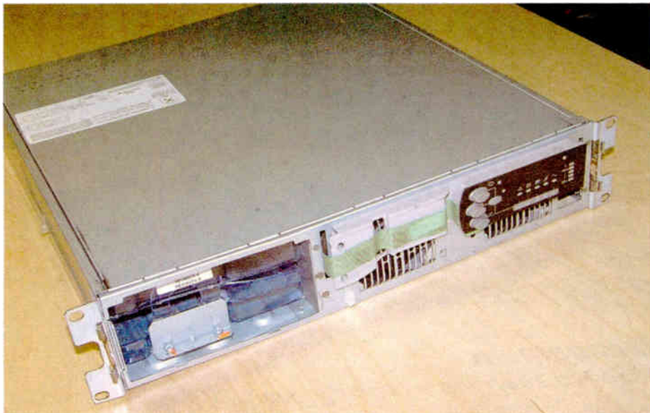
I found a Compaq R1500XR UPS on eBay, without batteries or faceplate. It was inexpensive. This is only one of many models that will suffice.
