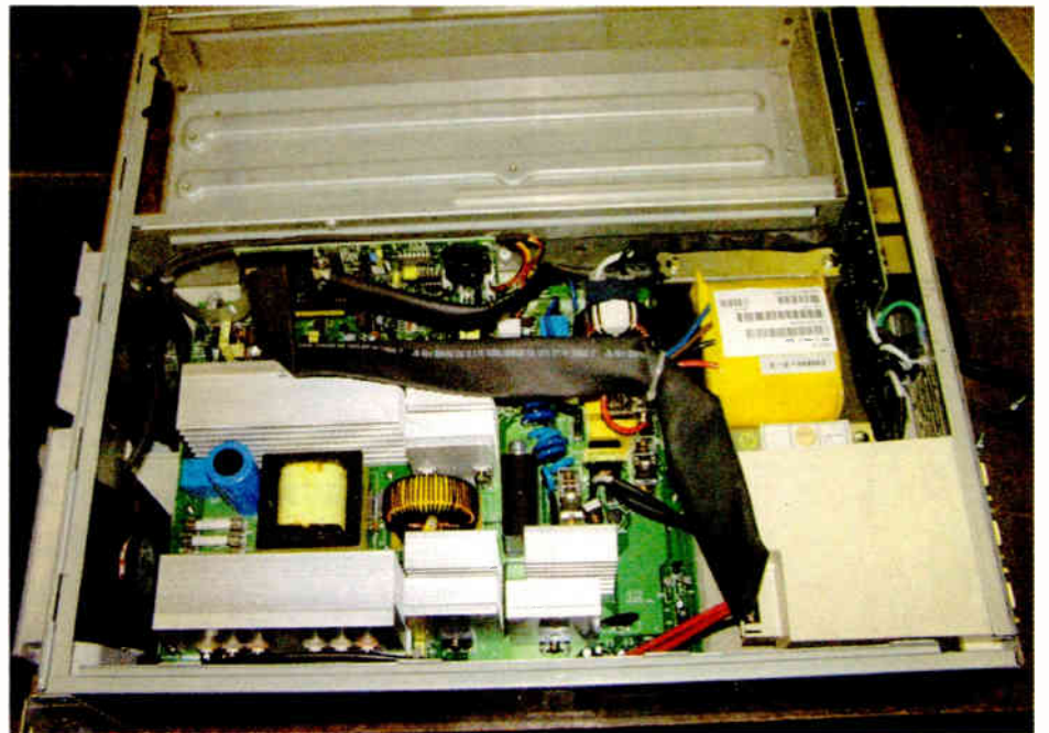
This is what it looks like with the cover removed. At the top is the empty battery compartment.
