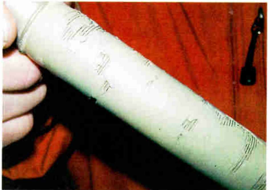
Fig. 2: Broken ceramic on wire-wound resistors usually indicates failure.
