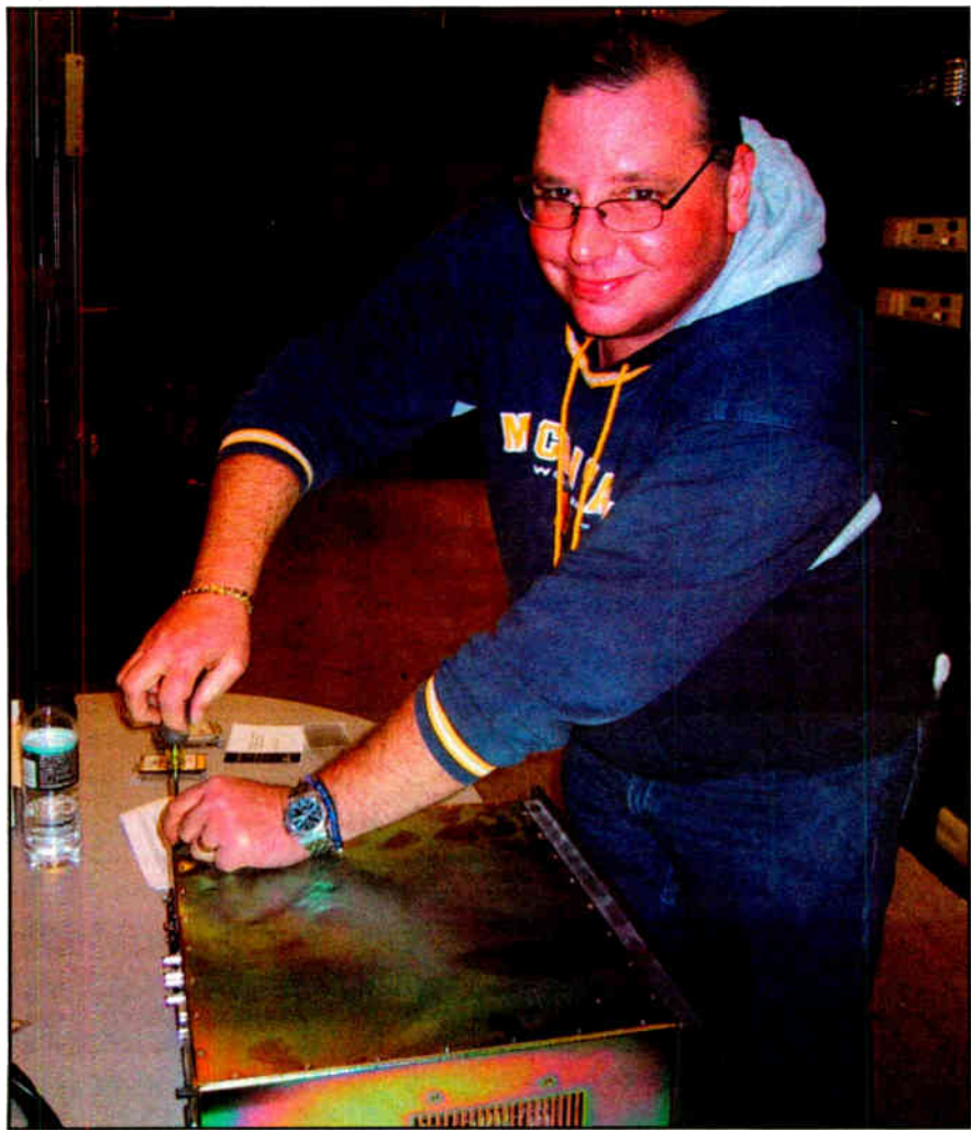
Tocco puts the cover back on the Omnia-6 after the firmware card replacement.
