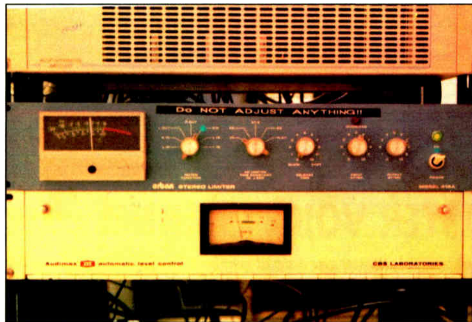
A mono Audimax is shown with a companion Orban 319. Note the gentle warning to passerby on the Orban.
