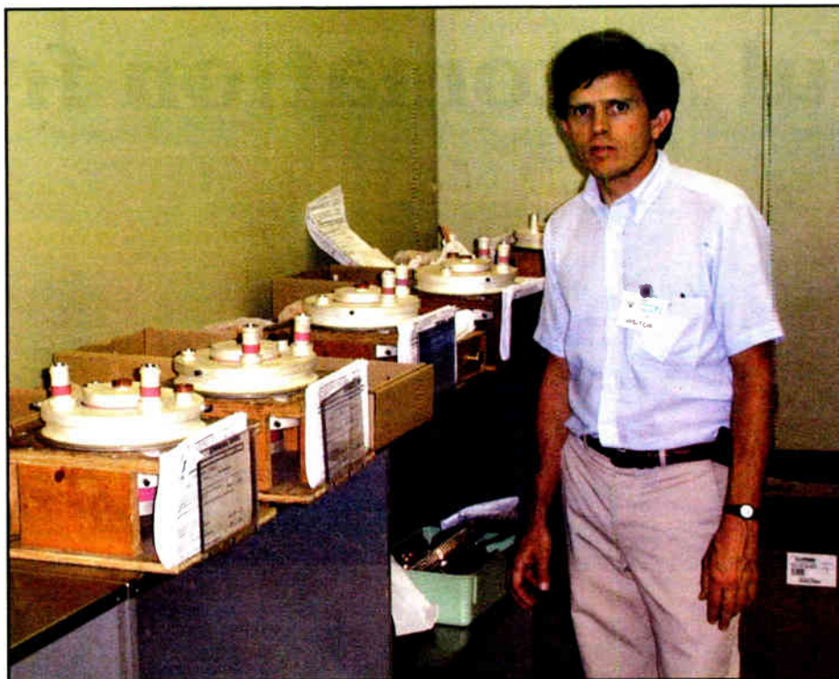
Fig. 3: John Lyles is shown with four rebuilt Burle/RCA 4616 tetrodes at the Burle Industries factory in Lancaster, Pa.
