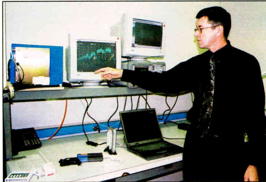
Steve Martin, FCC senior engineer, demonstrates BPL products, seen at lower left. The FCC has established some theoretical models and is testing field-strength theories related to BPL.
