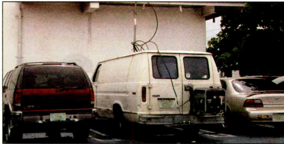
This was a mobile FM that used a generator and a push-up pole through the roof of the truck. Image has been altered to cover the license plate.
