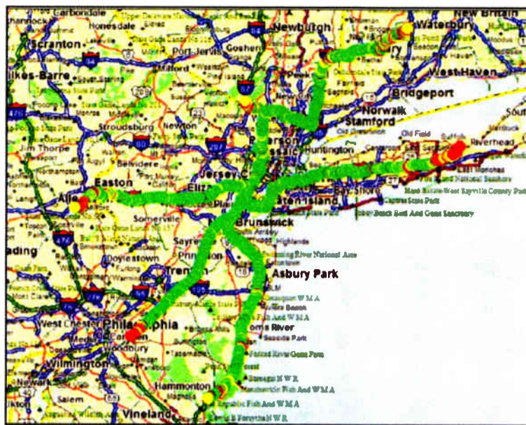
An Ibiqumy map predicts WOR(AM)'s digital coverage in green and yellow, blend-to-analog in red.
