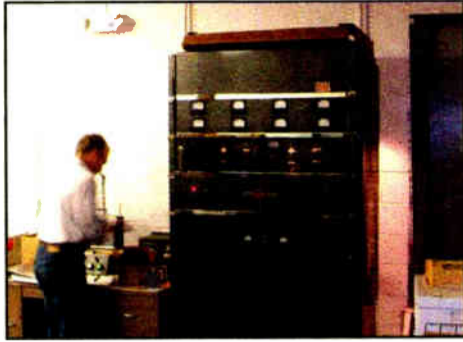
Engineer Tom Mackie, W2ILA, lights up the filaments on a quad of jumbo type-810 glass triodes in a vintage Collins broadcast transmitter.
