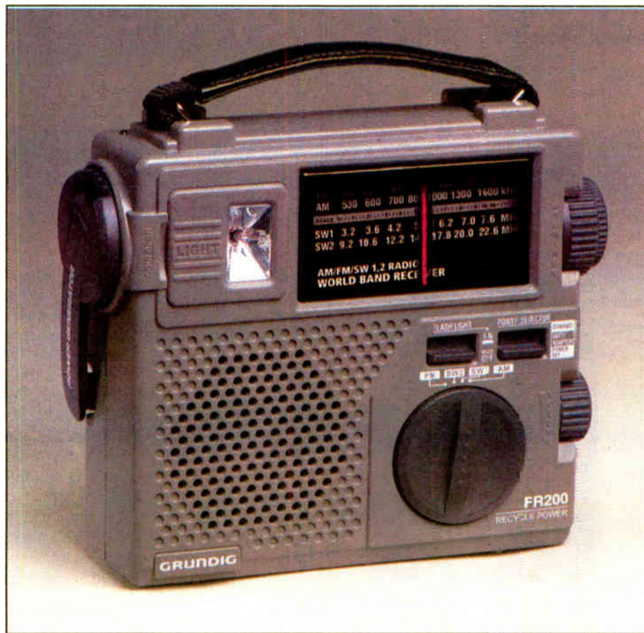
Eton's biggest seller is the FR200 receiver that includes an LED flashlight and hand-cranked generator that tops up its batteries.
