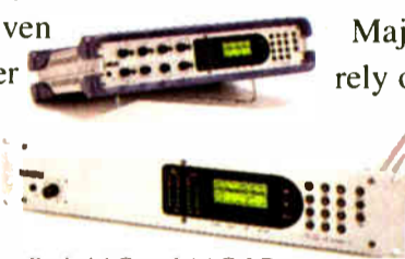
Both AAC and AAC-LD are featured in the Telos Zephyr Xstream rack and portable codecs.
