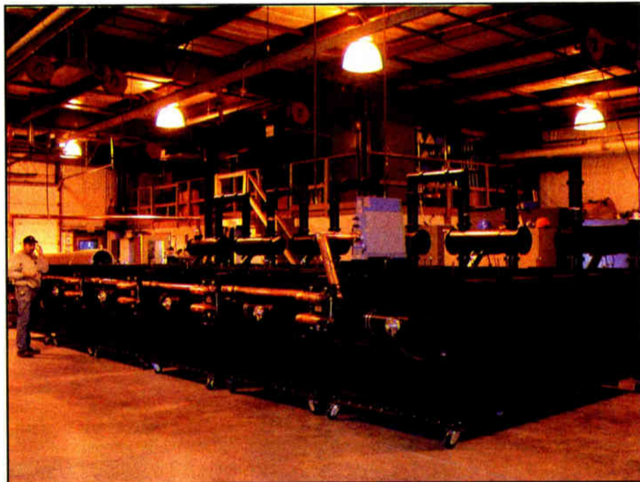
Dielectric workers build a six-station FM combiner at the Raymond, Maine, facility.
