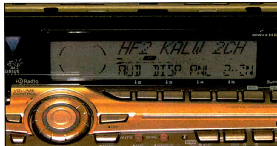
This Kenwood pre-production Tomorrow Radio head unit is shown tuned to a Supplemental Audio Program channel.
