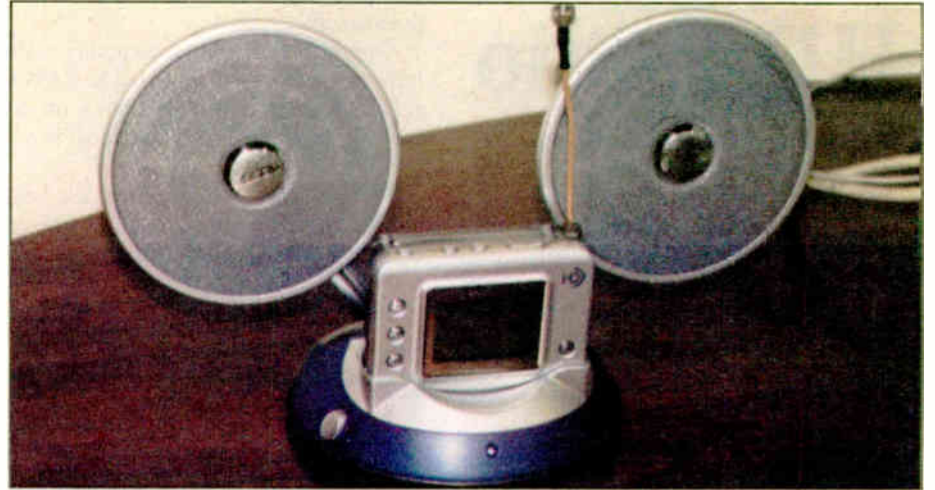
This portable HD Radio receiver from Personal Telecom comes with an MP3 player and FM tuner. The unit detaches from its docking station and can run on batteries for about an hour. When in the docking station, it can be plugged into the wall. The company showed a similar Eureka-147 version in the Texas Instruments booth.
