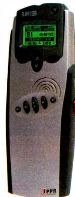
The Handheld II is a solid-state, MPEG-L2 recorder that fits in the palm.
