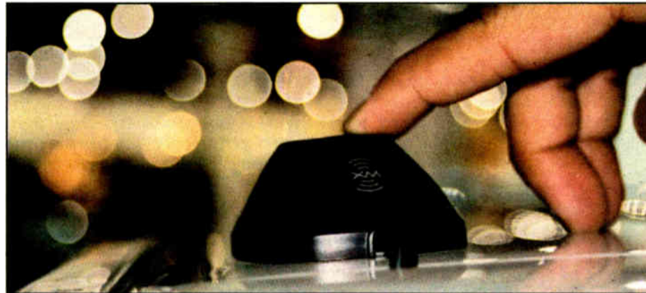
Antennas for XM and Sirius are getting smaller. This is a roof-mounted XM antenna.
