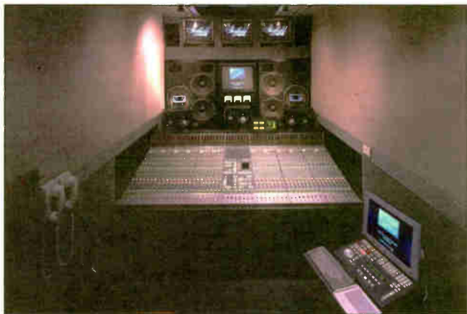
The Sheffield Remote Productions 48-foot remote truck uses an SSL Axiom-MT Digital Console and has 10-foot ceilings, lead-lined walls, sand-filled floors and an elevated client lounge and vocal booth.
