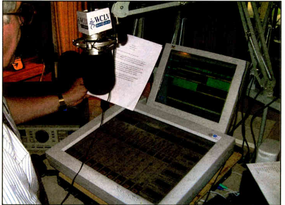
In the talk studio, the station uses Logitek vMix software, controlling a Digital Audio Engine from a computer screen.
