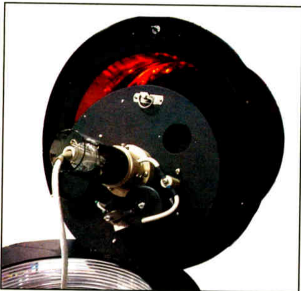
Fig. 2 shows the flash tube in the lower part of a dual flash tube strobe light, which provides the white beacon for daylight operation.
