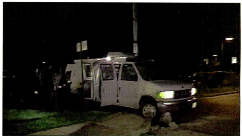
A crew from WTTG(TV), Washington ran its van mast into a 230,000-volt circuit line in 2000. The mast transferred 115,000 volts to the ground, lifted rocks and shattered the sidewalk and curbing within seconds. The photographer had a camera on his shoulder, tethered to the truck with multiconductor cable. It exploded. He has not returned to work two years later due to his injuries.
