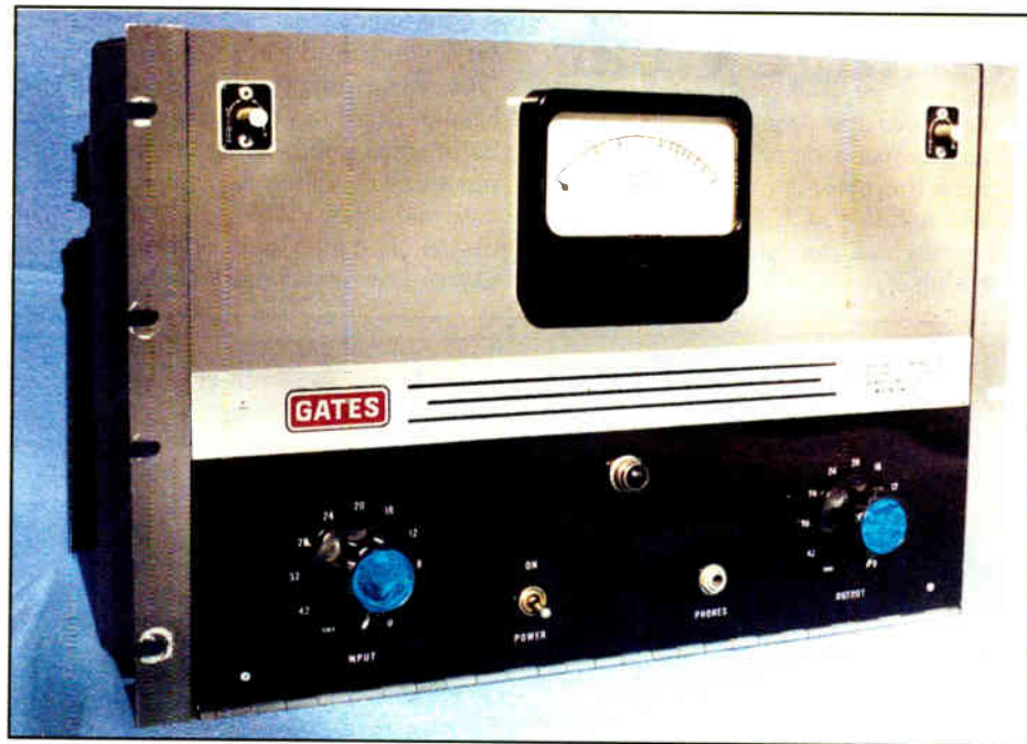
This Gates SA-39B peak limiter once processed beautiful music for a Boston radio station.
