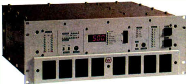
Some AM stations wish to use FM translators like this one from Crown Broadcast.
