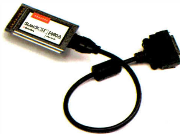
The Adaptec SlimSCSI 1480 achieves nearly triple the throughput of its 1460 PCMCIA card.
