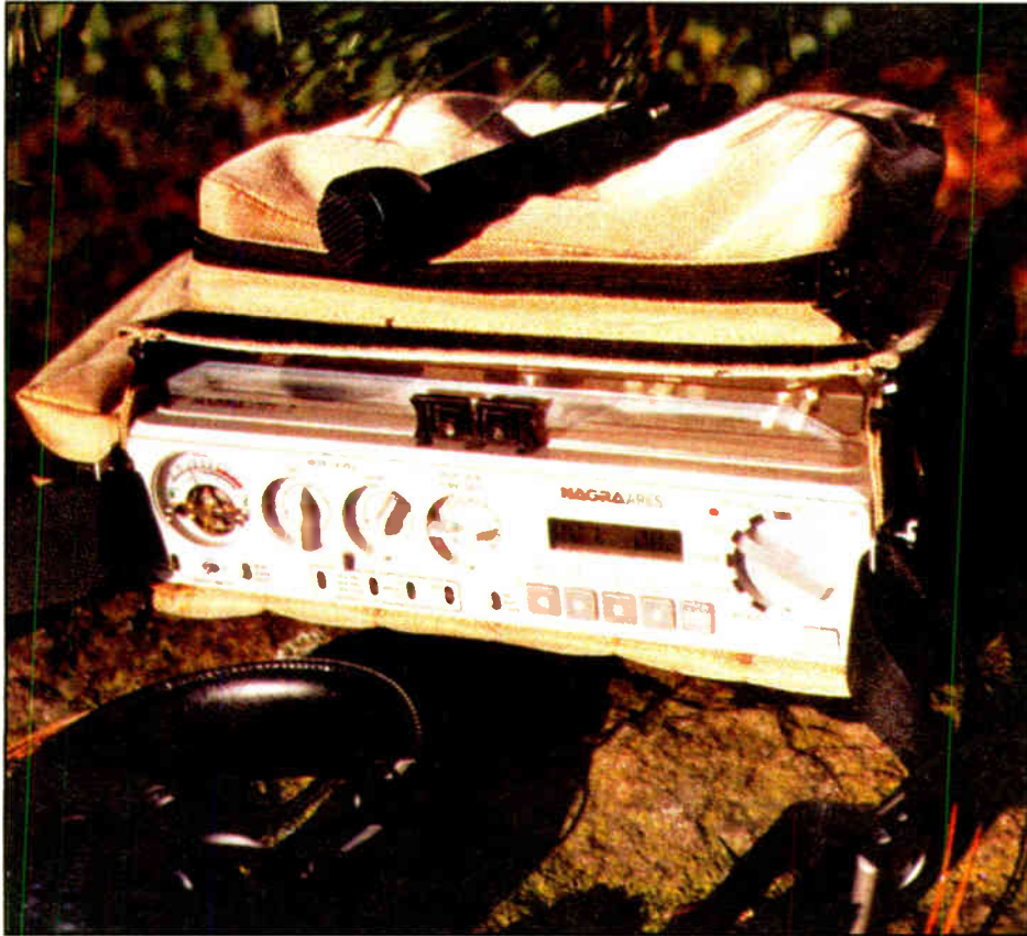
The Nagra ARES digital recorder uses PCMCIA RAM media.
