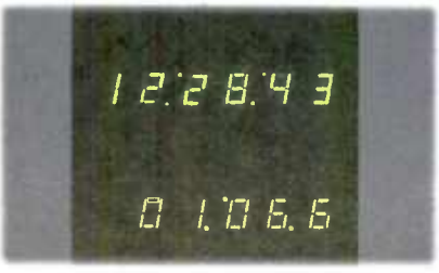
The digital timer displays the tenth-of-second digit in the Hold and Stop modes, but blanks it when time is running to minimize distraction to the board operator.
