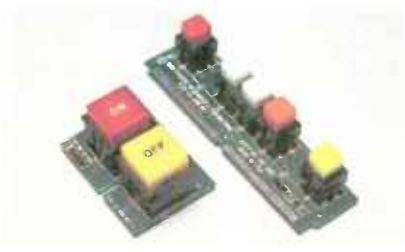
Sealed, LED illuminated buttons are designed so you can remove the switch assembly without unsoldering, in case of a coffee spill.
