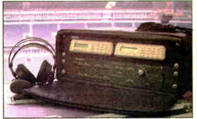
MIDCOM's ISDN rack uses Adtran TAs to interface ISDN with the CCS codecs.
