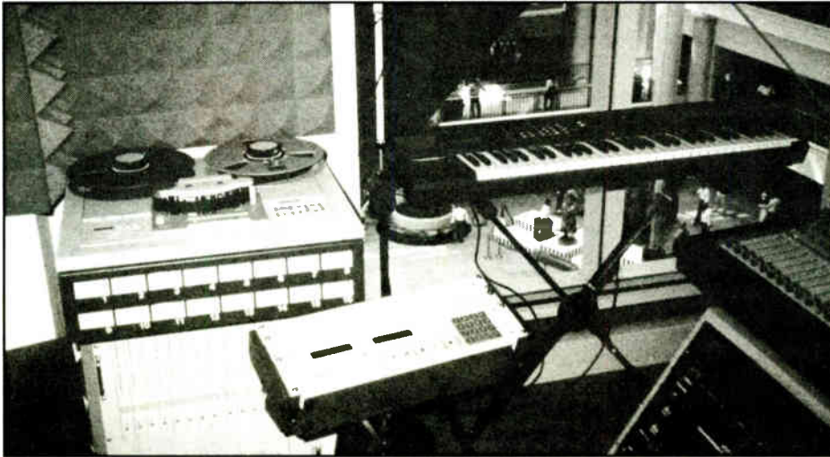
WMMS(FM)'s Zoodio comes equipped with a 16-track Tascam reel-to-reel and an arsenal of processing gear.
