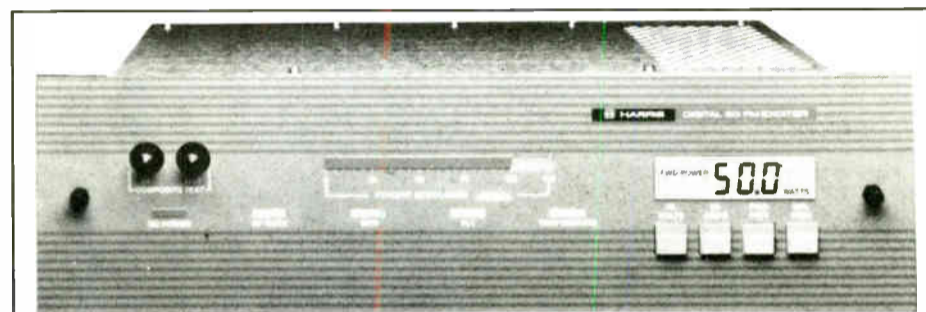
Harris Digital 50, 50 Watt digital solid state FM exciter
