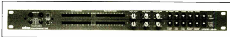
Orban's Co-Operator controls the audio signal from WILL's five studios to its transmitter.
