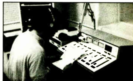
The station's newsroom features an Autogram Pacemaker console, BE cart machines and a Tascam reel-to-reel.
