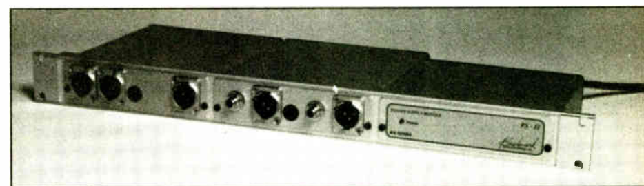
The PS-11 power supply is part of Benchmark Media Systems' IFA interface amplifiers.
