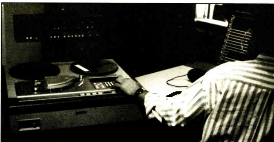
Synchronization for the simulcast was accomplished with the help of MPR's Sony PCM-3402 DASH recorder.
