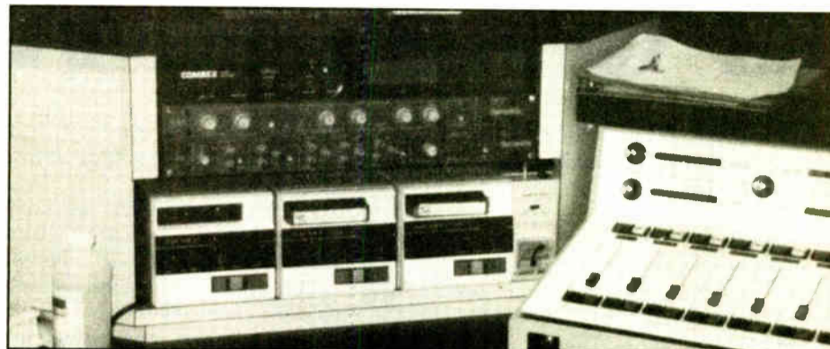
BE Dura Trak 90 and Phase Trak 90 cart machines play back commercials in the control room at KTMJ.
