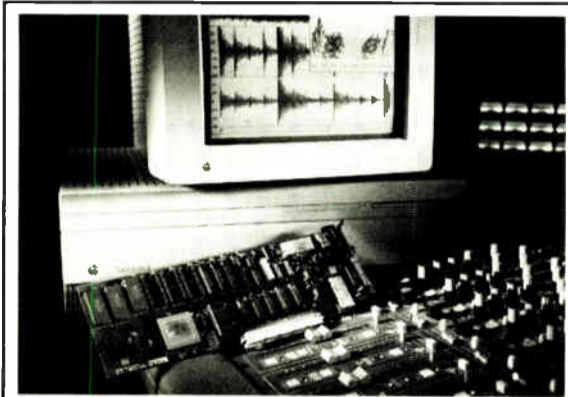
Digidesign's Sound Accelerator™ card allows an Apple Macintosh II to be used as an audio workstation.
