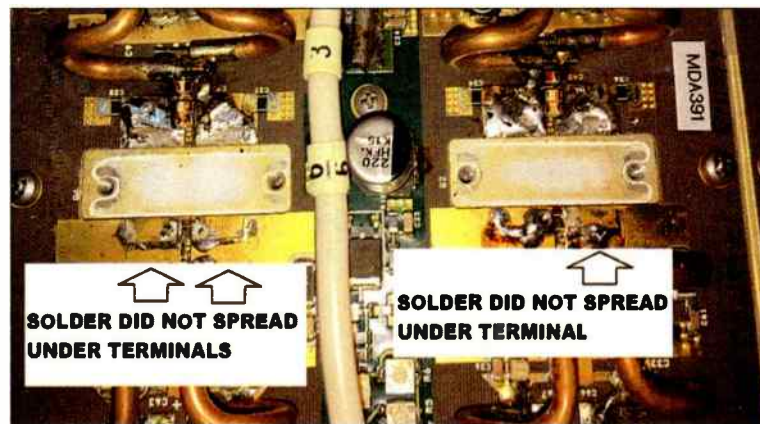
Figure 2: With the FETs taken off, we noticed that there was no solder under the gate leads. There was also one solder joint that cracked. Thankfully, it worked fine after we re-soldered the joint.
