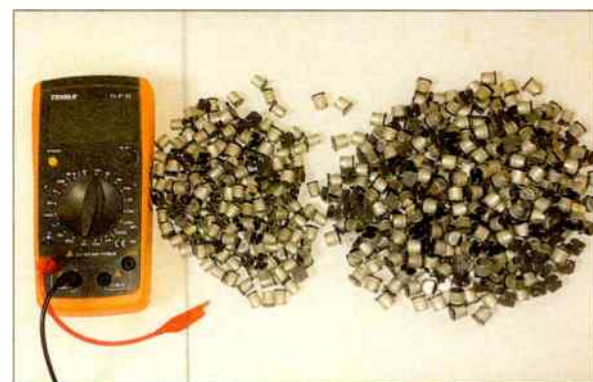
All the old surface-mount capacitors were replaced with a higher voltage rated capacitor. The bunch on the left are 35V rated while the 50V ones are on the right side.
