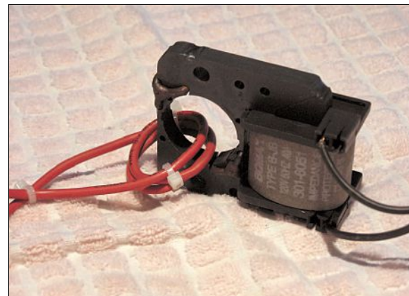
Repurposing an old motor as a current transformer.
