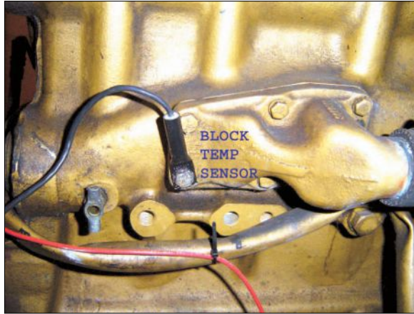
Temperature sensor is bolted to the engine block just above the block heater output pipe.
