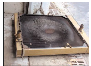
Dirty air and oil leaks can rapidly deteriorate the heat dissipation capability of a radiator.
