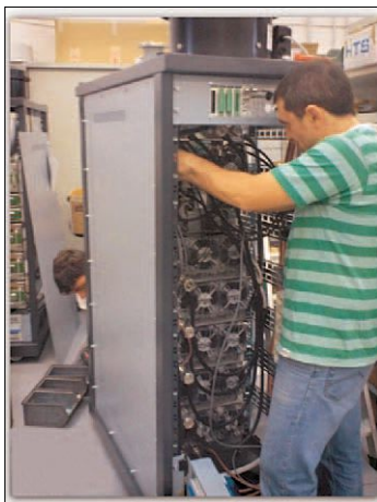
Final assembly of a high power solid state transmitters.
