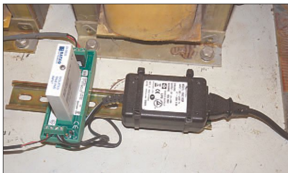
A Dataq module installed in a Harris 3.5K, used to monitor the filament voltage.
