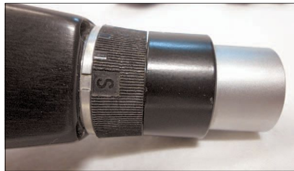
The bass roll off switch on the MD421U.
