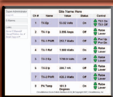
Internal Web Server
