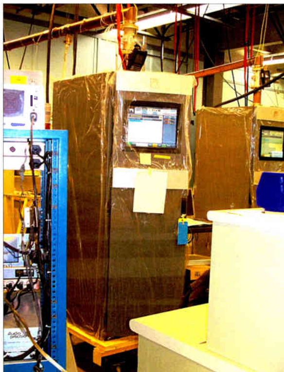
An NV Series transmitter going through Nautel's testing and burn-in before shipment. Note the unit is covered in plastic to help avoid scratches to the transmitter's finish. Nautel has a reputation of paying attention to even this smallest of detail.
