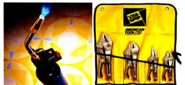
A torch and vise grips come in handy when dealing with copper strap, etc.
