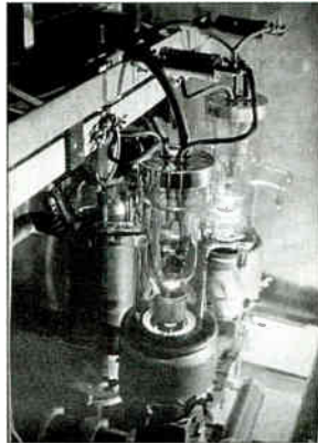
UV862 tubes in operation.
