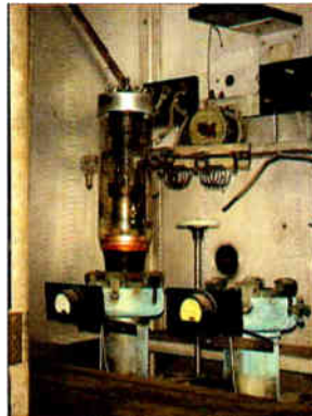
A UV898 tube in its socket today. Notice the disconnected filament leads at the top.
